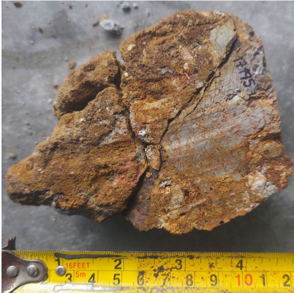
Figure 4: Polymictic mineralized breccia sample grading 7.1 g/t Au from channel CH17191 (96.5 m @ 0.6 g/t Au) Previsto Central, showing angular clasts set in a oxide-after-sulphide-bearing cement of potassium feldspar, quartz and carbonate, a texture characteristic of the alkalic porphyry-epithermal system.
