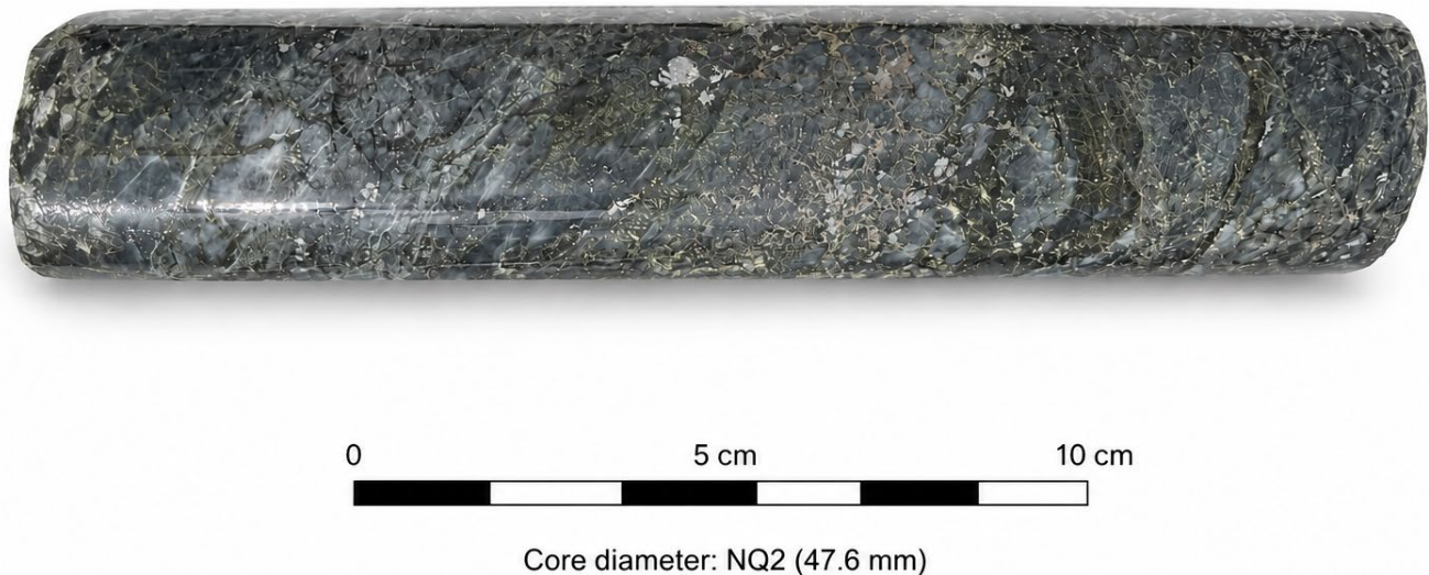
Photo 1: Core sample from ST2601 at 80.48 m showing arsenopyrite, pyrrhotite and chalcopyrite in a quartz shear vein, returning 8.9 g/t Au, 47.5 g/t Ag and 0.74% Cu.
