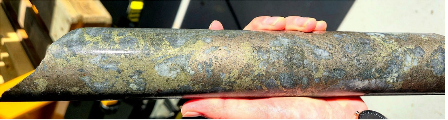
Plate 1: Core sample from ST2606 at 80.9 m showing chalcopyrite, pyrrhotite and arsenopyrite in a quartz shear vein, returning 0.4 m @ 6.5 g/t Au, 66.4 g/t Ag and 1.35% Cu. Core size is NQ2 (diameter 55.6 mm).
